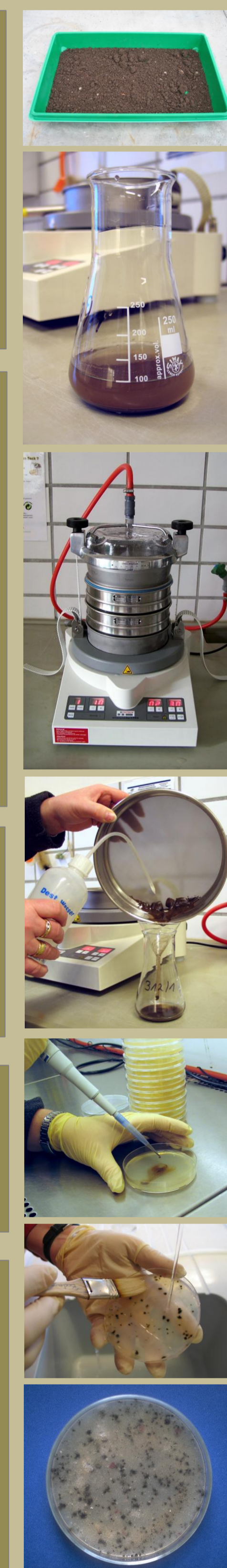
Fig. 1: Standardized wet-sieving and plating method used in German labs for quantitative detection of Verticillium in soil.
